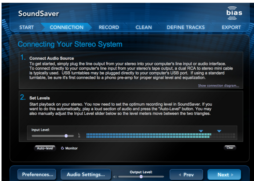
The Connection page helps you connect your audio source to your computer, and to set an optimal recording level.
