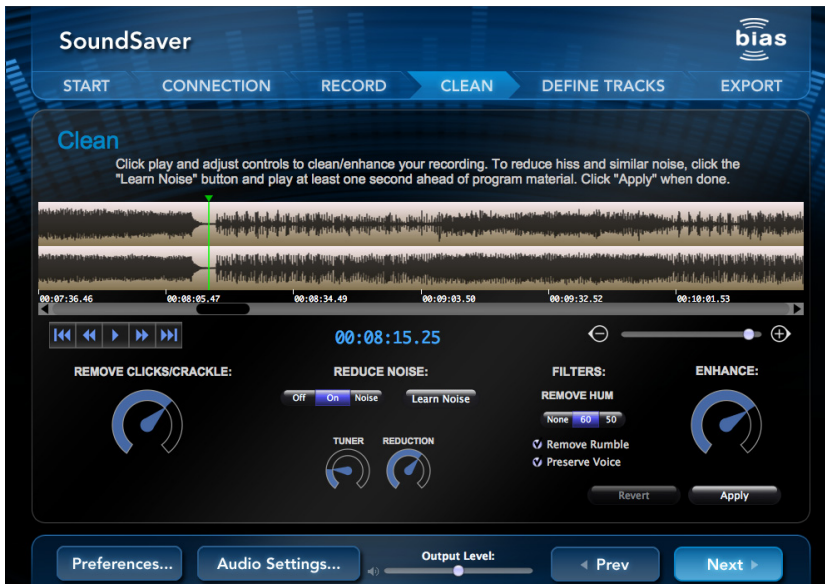
The Clean page is where you can remove unwanted noise from your recordings – SoundSaver can remove clicks, crackles, pops, hiss, hum, and rumble, all of which are commonly found in recordings made from records and cassettes.
